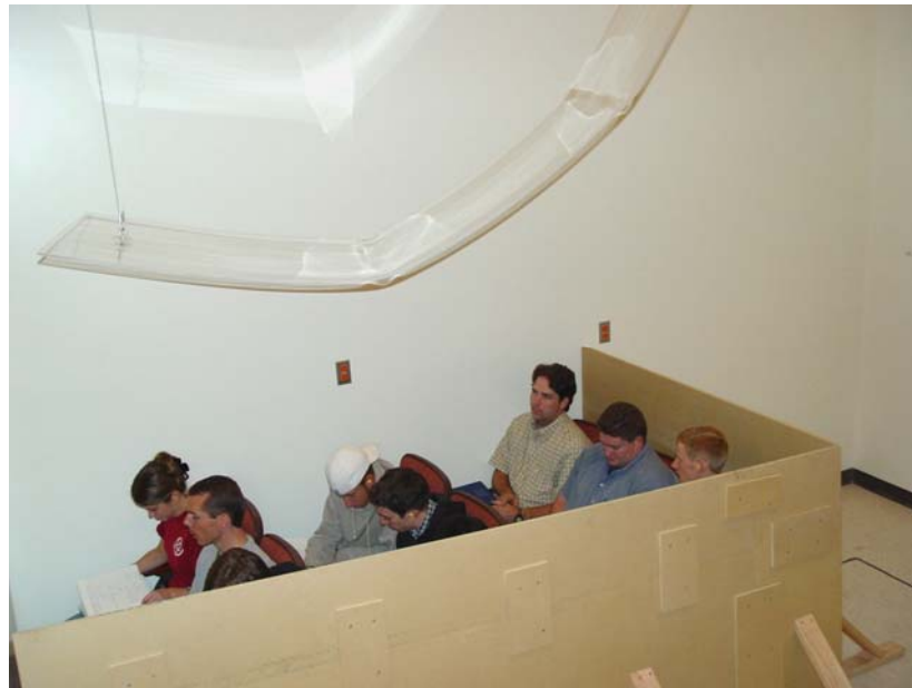
Figure 6.9. Setup in the reverberation chamber for measuring the audience absorption.
