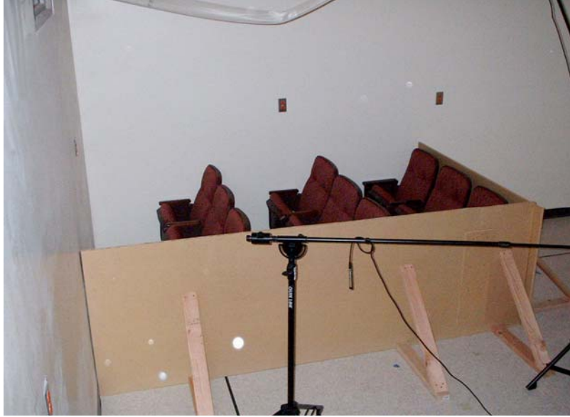
Figure 6.6. Setup in the reverberation chamber for measuring the absorption of empty chairs.
